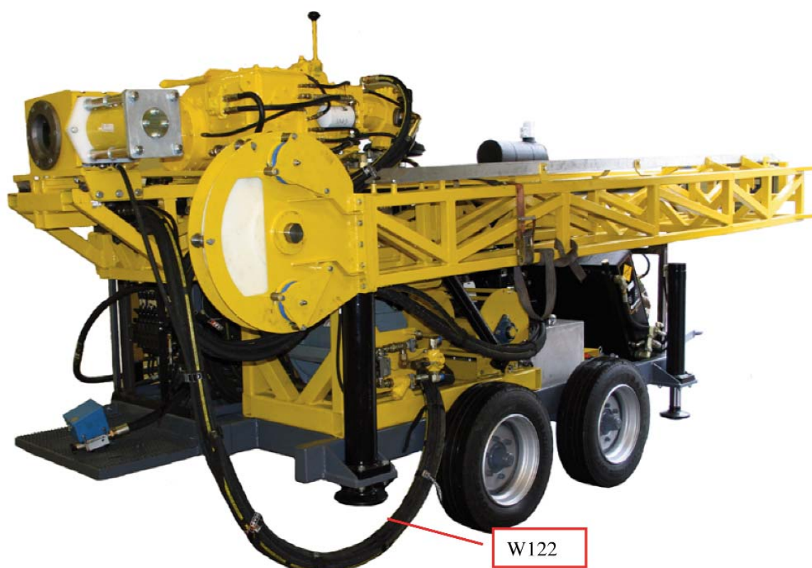
Fig2: Cable from Transmitter to Tachometer from feed unit to rig along the hydraulic hoses.
